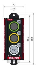
The superior system connects to the device's M12 connector CAN-in via a gateway and CAN bus. The unit draws power from the same connector.
