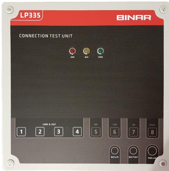
Picture: LP335 – CTU (Connection test unit)
