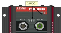
The Yellow BUS illuminates when the Gateway establishes communication with the device, which typically occurs immediately following power-on and remains continuous thereafter. The red ERR signals an error on the device.
