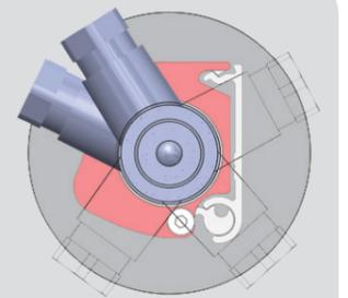
The M12 connection plug can be rotated. A connected M12 plug can therefore be angled arbitrarily within the green area as shown on the picture above. By doing this, the outgoing cable can be located at a suitable direction.
